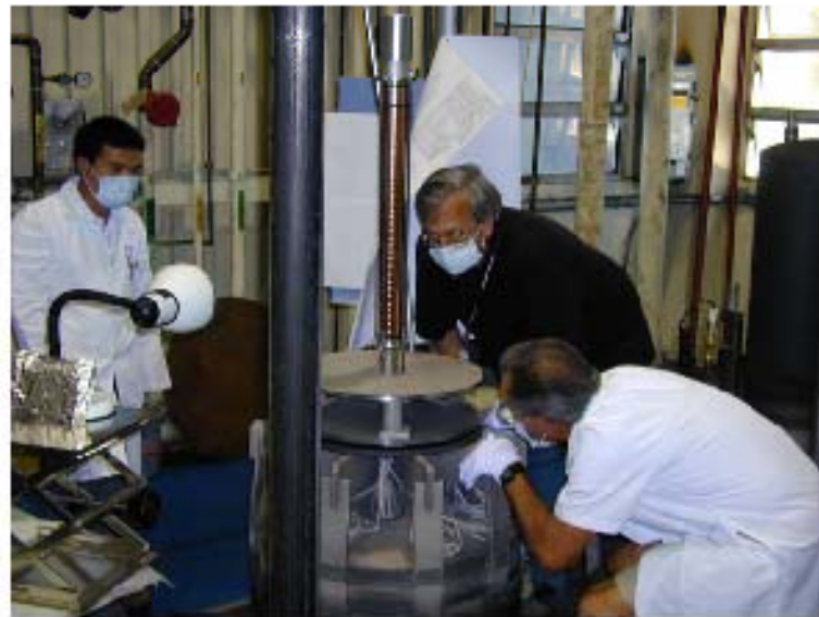
Supports for the Lower Plate are Carefully Removed. Its Weight is Then Transferred to the Top of the Structure Through the Three Rods.
