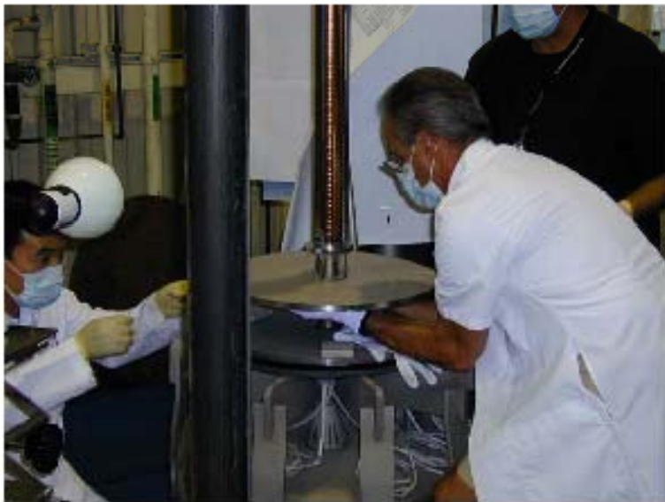
Supports for the Lower Plate are Carefully Removed. Its Weight is Then Transferred to the Top of the Structure Through the Three Rods.
