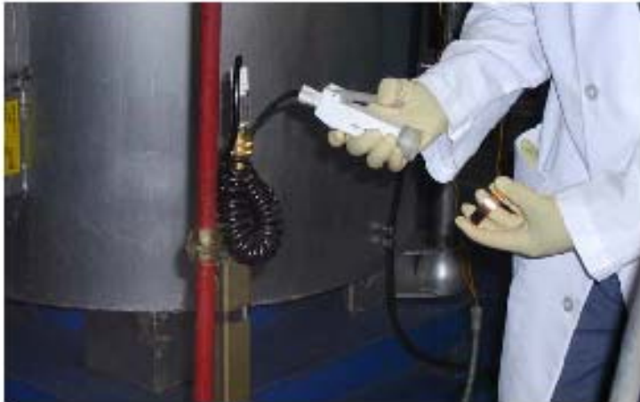
Sometimes Pressurized Filtered Nitrogen Is Used to Remove Particulates from a Cell.
