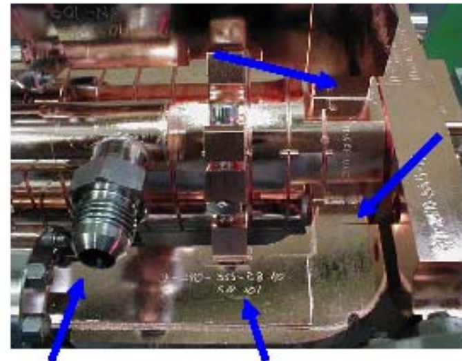
Water fitting for structure cooling
