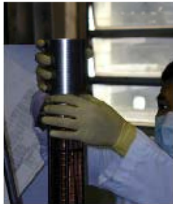
Once the Rods are Inserted, a Temporary Weight Prevents Shifting of the Cells.
