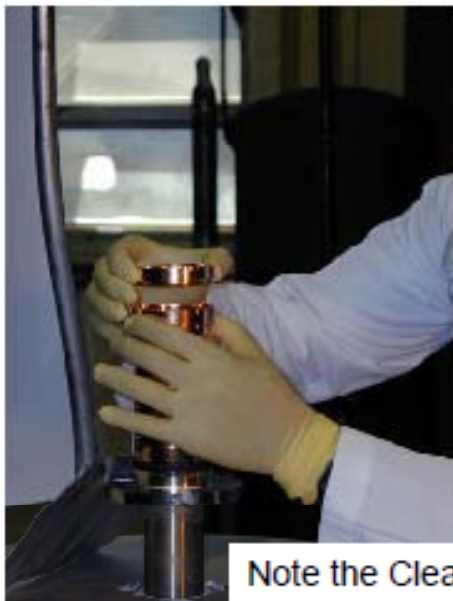
Both Rotational and Vertical Alignment are Checked to the Limits of the Transit – a Few Mils.
